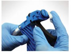
Apply a small amount of petroleum jelly to the ring surrounding the face of the gun before attaching the nozzle.
