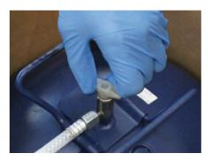
Open valves fully and check flow by pulling the trigger and dispensing into a waste container before attaching a nozzle.
