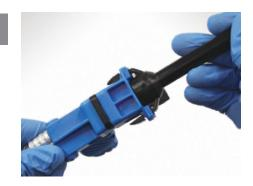
Line up the arms of the nozzle with the slots in the gun and push firmly until you hear a click.
