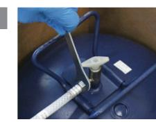
Shake both tanks for 1-2 minutes before use. Attach the A and B-labeled hoses to their corresponding tanks. Hand tighten and secure with a wrench. DO NOT over tighten. 2
