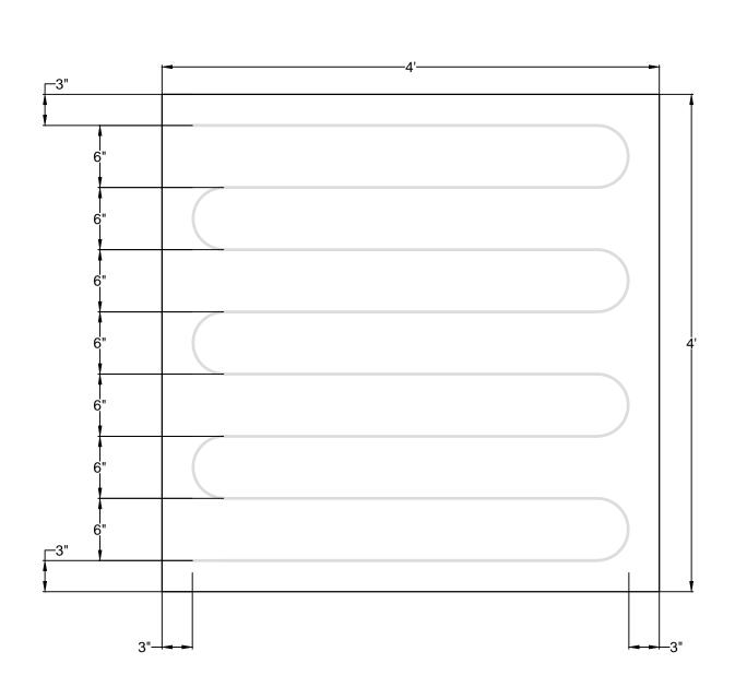
ADHESIVE APPLIED IN A CONTINUOUS 3/4" TO 1" WET BEAD MAXIMUM INSULATION BOARD SIZE: 48" X 48" MAXIMUM BOARD THICKNESS 2.7' PER LAYER
