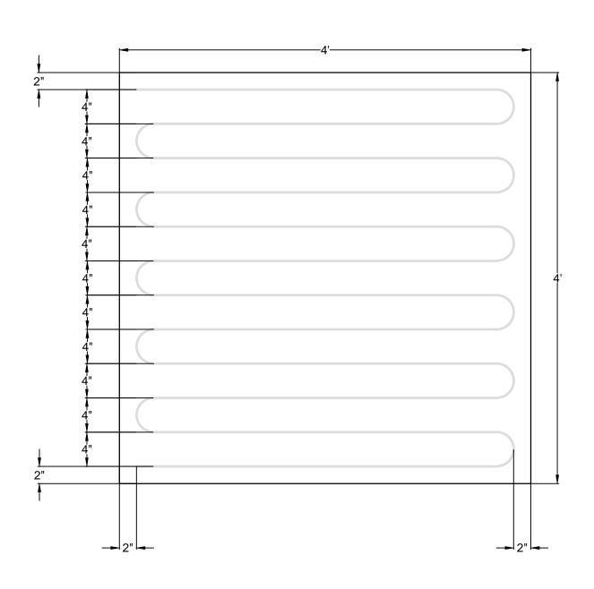
ADHESIVE APPLIED IN A CONTINUOUS 3/4" TO 1" WET BEAD MAXIMUM INSULATION BOARD SIZE: 48" X 48" MAXIMUM BOARD THICKNESS 2.7" PER LAYER
