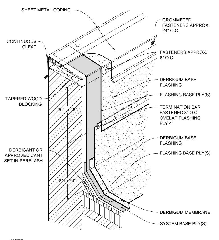
NOTE: THIS DETAIL SHOULD ONLY BE USED WHEN THE DECK IS SUPPORTED BY THE WALL.
