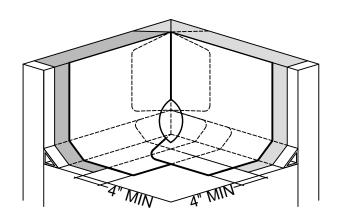
NOTES: INSTALL BOOTS ON ALL CAP AND BASE PLY BASE FLASHING CORNER AS SHOWN..
