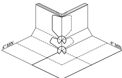
NOTES: INSTALL NOTCHED (SHOWN) OR BOWTIE BOOTS ON BASE AND CAP FLASHING CORNERS.
